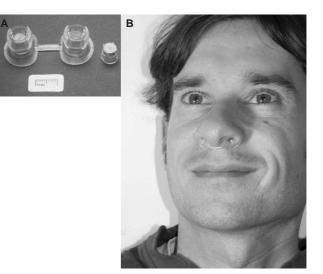
**Figure 2.** (A) Intra-nasal air sampler. Disassembled components for the intra-nasal air sampler, a soft silicon strap spans the septum of the nose and connects the two silicon frames that house the collection cups. (B) Fully assembled intra-nasal air sampler worn by a subject.
